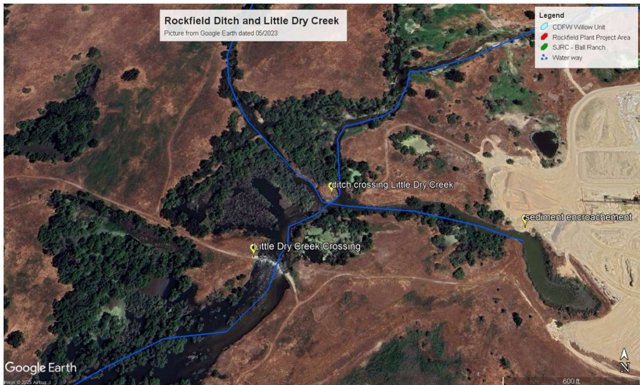
Figure 10: Rockfield water supply ditch with a focus on the crossing of Little Dry Creek and the inlet pond from Google Earth, access in March 2025 and using the time series tool to show May 2023. Note that Little Dry is flowing and that the surface disturbance at the plant site goes up to the inlet pond, allowing siltation and contaminants to enter the inlet ditch waters that are connected to Little Dry Creek.
