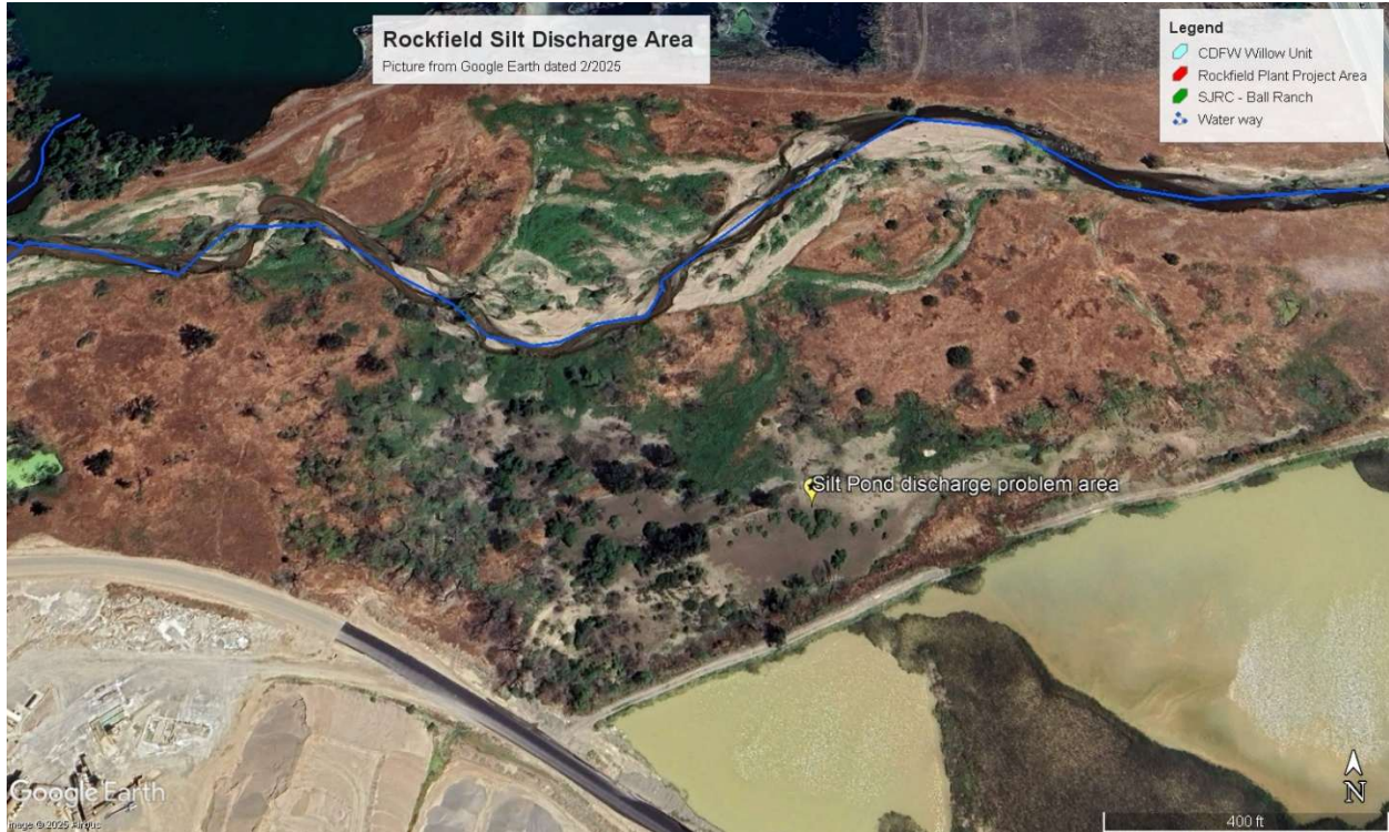
Figure 4: Google Earth Image from March 2025 showing existing conditions with a focus on the silt pond and Little Dry Creek. Note the silt deposits next to the silt pond.
